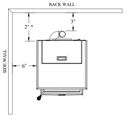
Figure 1 Back wall installation
